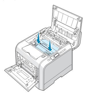
**12** Firmly push the lock levers on each side towards the top cover, as shown below, to lock the transfer belt into place.
